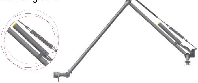
The Long-Reach Bottom Loading Arm is a long reach bottom loading arm that is ideal for extended reach bottom truck loading spots, particularly where "B-Trains" or double length trailers are being loaded. The MYR excels at long reach loading with an effective working reach ranging from 6' to 18' and a connection height envelope from 24" – 54". Not recommended where multiple arm cross-over is required.
