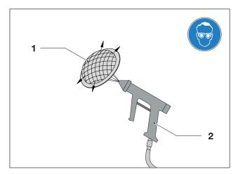
Fig. 11 Blowing out the mesh filter
