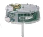
The VSM valve is also equipped with a special PSM pilot valve fitted on the lid, which also makes it work as a relief valve in pressure, with a maximum over pressure 5% lower than the setting pressure.
