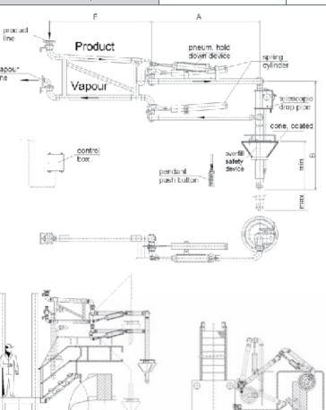
The E2632 is the technically best solution for the loading process with vapor return. Due to the vapor line without slop, collection of condensate is prevented. The design allows heating of product and vapor line. The design of the vapor line with swivel joints gives an easy handling as a further advantage against the use of hoses.
