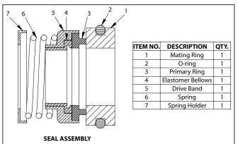
inspect the lapped sealing face of carbon washer (Part 3) for wear which would necessitate replacement.
