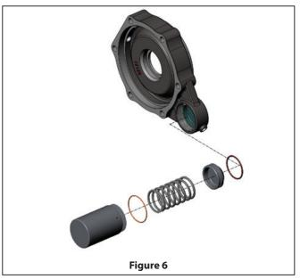
Continue filling seal cavity until high-pressure grease reservoir is full. **NOTE**: When grease reservoir is full it will spit out of the pressure release valve.
