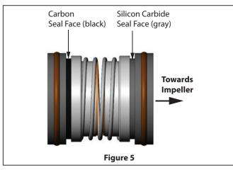
Install seal spring over drive sleeve onto backside of silicon carbide seal. Apply P80 to interior seal bellows of carbon seal and push over drive sleeve with seal pusher carbon face up. Inspect and wipe clean, if necessary. Install gasket over studs onto seal housing. Apply P80 to seal seat bore of adapter and around O-ring on seal seat. Push seal seat, by hand, into seal bore – clean and inspect.
