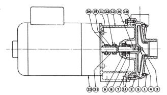
sealer such as Permatex between outside diameter of seal head and casting bore. When shipped from factory, the seal head is usually pressed in place already.
