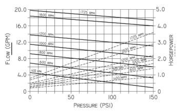
\* For pressures over 100 p.s.i., the above selections are suitable for pumping fluids with lubricity (eq. oils, polymers). Service life will decrease for fluids without lubricity (eq. water, solvents).
