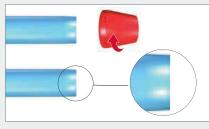
1. Remove burrs from the outside diameter of the tube. Clean and remove any shavings.
