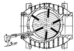
Fig. 7.5 Check rotor vanes for height wear
