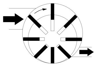
Functional principle of a rotary compressor or a compressor and vacuum pump
