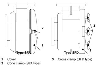
Fig. 7.1 Vacuum filter SFA and SFD
