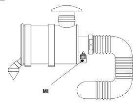
Fig. 4.7 Combination air filter/maintenance indicator
