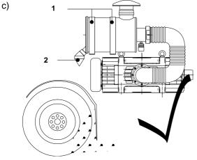
fig. 4.5 Installing the combination air filter
