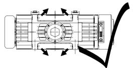
fig. 4.8 Air cooling system
