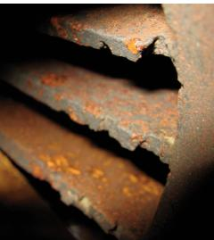
Effects of cavitation on a rotor taper bore
