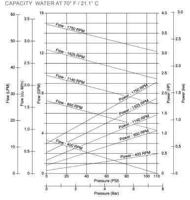
Notes: For continuous service: Plastic / Plastic gear combinations are limited to 50 psi or 3.5 bar. Metal / Plastic gear combinations are limited to 100 psi or 7 bar.
