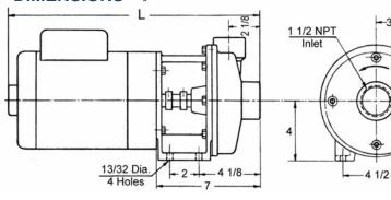
\*"L" Dimension for Single phase motors is 18 1/2"; for Three phase motors, it is 17 1/2"
