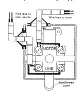
406MK-04N26 is supplied in the "Factory Supplied" CCW rotation orientation shown on pg.3 and with the vacuum switch prewired to the 1 HP motor for 115 V operation. A convenient 8 ' long power cord and plug is provided.
