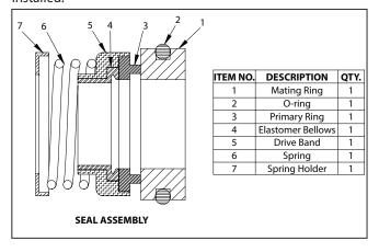
inspect the lapped sealing face of carbon washer (Part 3) for wear which would necessitate replacement.
