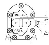
/ GREASE FITTINGS (ITEM 19) INSTALLED INTO .125-27 NPT CONNECTIONS.
