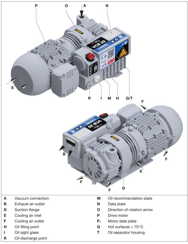
Fig. 2 Vacuum pump V-VCB
