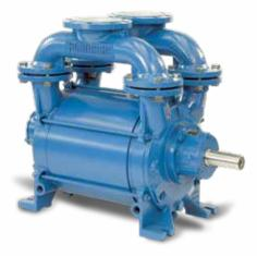
The **RVS** series are liquid ring vacuum pumps and thanks to innovative features, they are able to suck in gas and vapors, without contamination from lubricants, even with dragged fluid and virtually isothermal gas compression. The series can achieve up to 33 mbar (a) and capacity up to 4200 m<sup>3</sup>/h. Thanks to its construction characteristics, the liquid ring vacuum pumps are renowned for low water consumption, minimum noise level and vibrations, reliable service and easy maintenance.
