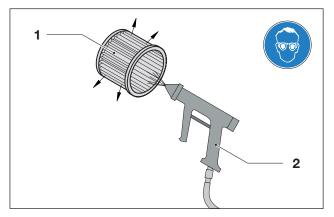
Fig. 4 Purging filter cartridge
