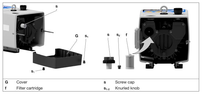
Fig. 4 Replacement of air filter
