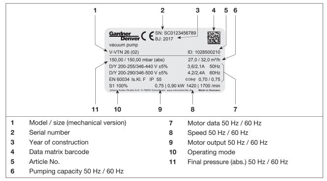
Fig. 3 Data plate (example)
