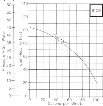
and are wired for the proper pump rotation which is counter-clockwise looking at inlet end of pump. See the dimensional drawing on back. Three phase motors must be checked out for proper rotation when pump is installed. Interchanging of any 2 wires in a 3-phase system will reverse motor rotation.
