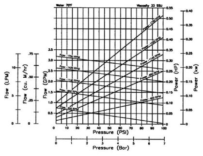
Notes: For continuous service: Plastic / Plastic gear combinations are limited to 50 psi. Metal / Plastic gear combinations are limited to 100 psi. Horsepower requirements increase for viscous fluids.
