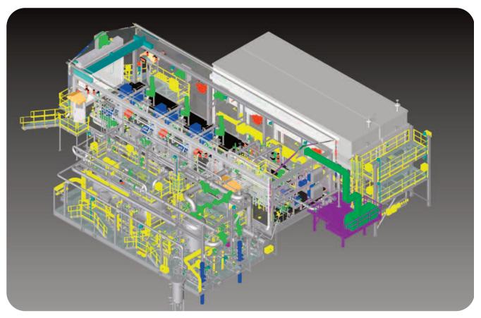
Design drawing of a complete ETO system constructed at the North America Manufacturing location. Project consists of multiple skids, weather proof enclosure with power, heat, lights; multi level tank skid, heated weather proof connections; and two air coolers.
