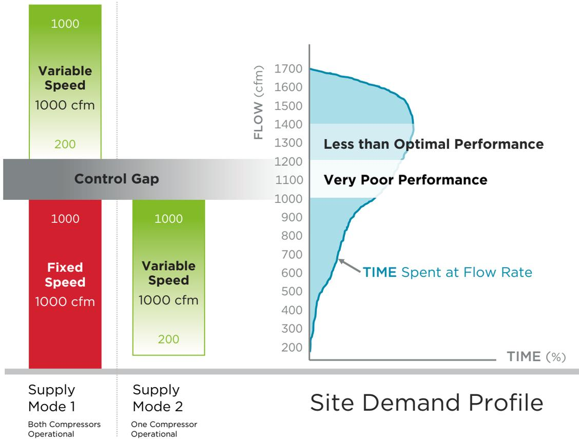
Control gaps commonly exist in compressed air systems, especially when the variable speed (VS) compressor is the same capacity as the fixed speed compressor.
