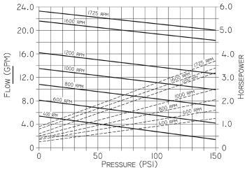
\* For pressures over 100 psi, the above selections are suitable for pumping fluids with lubricity (eq. oils, polymers). Service life will decrease for fluids without lubricity (eq. water, solvents).
