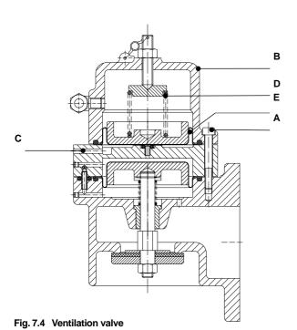
To avoid this carry out a visual check of the ventilation valve regularly (at least every 3 months and, if necessary, dismantle the ventilation valve, clean the dirt and blow out the bore hole for pressure compensation with compressed air.
