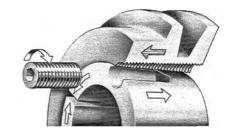
2. Push the disk with the bush onto the shaft, align it and tighten the screws evenly and tightly.
