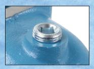
A fill port added to the housing for ease of pre-filling the priming chamber.
