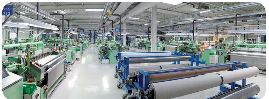
Almost all the machines and equipment for metal mesh production at GKD require compressed air as energy and/or as transport medium.
