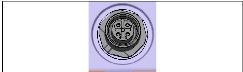
Round connector, 5-pol., M12, B- encoded for fieldbus profibus
