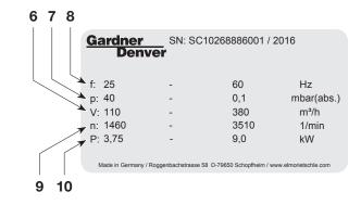
Fig. 5 Data plate of the frequency converter
