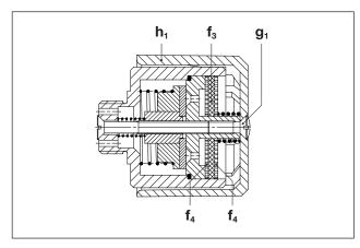
Fig. 12 Gas ballast valve
