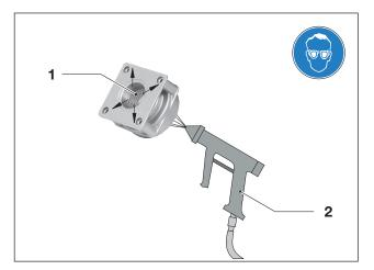
Fig. 13 Blowing out the mesh filter
