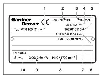
Fig. 4 Data plate (example)
