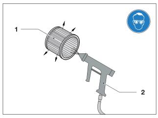
Fig. 6 Purging filter cartridge
