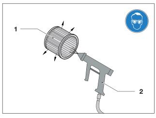
Fig. 8 Purging filter cartridge
