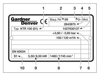
Fig. 3 Data plate (example)
