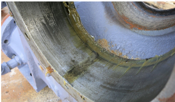
The ‘Other’ Shop did not address visible wearing to the bearing bore. The part is out of spec, and will not perform efficiently.
