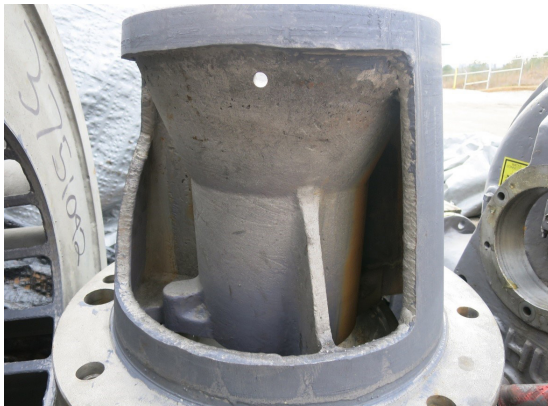
The ‘Other’ Shop returned the pump to the customer with a visibly worn cone surface, and cone tip measurements that do not meet spec.
