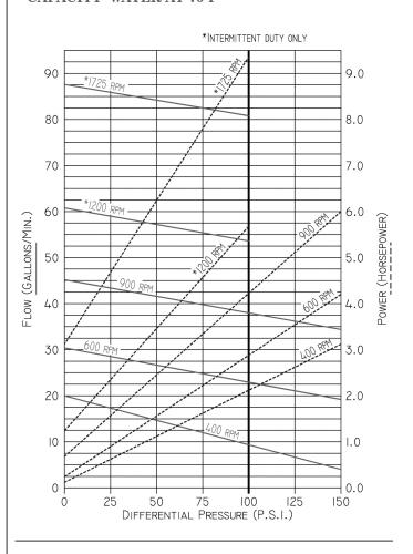
900 RPM not recommended except for intermittent duty and pressures below 100 psi.
