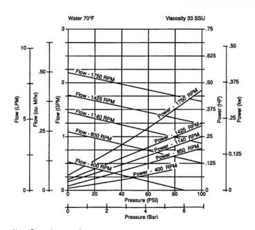
Notes: For continuous service: Plastic / Plastic gear combinations are limited to 50 psi. Metal/Plastic gear combinations are limited to 100 psi. Horsepower requirements increase for viscous fluids
