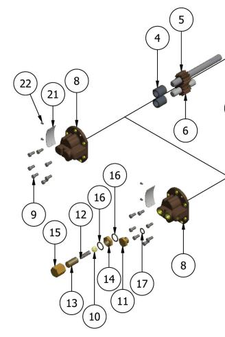
Items 8 and 10-17 for the "R" versions only. Item 23 is only used on N1000S5 pumps. Item 20 is only used on N1000S8 pumps.
