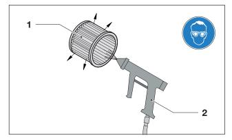
Fig. 10 Purging filter cartridge
