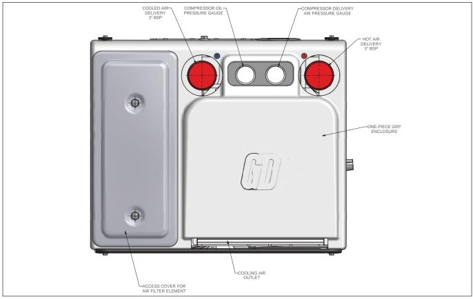
Figure 2a - Components Front View Clockwise (Right Hand) Rotation
