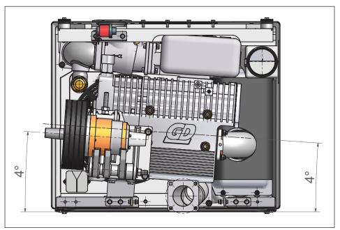
Figure 5g - Bulkline & Pulley Package Mounting Arrangement
