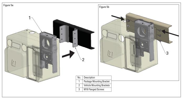
Figure 5 - Installation of Bulkline 650/1000 LNC Package to the Vehicle Mounting Bracket/Chassis
