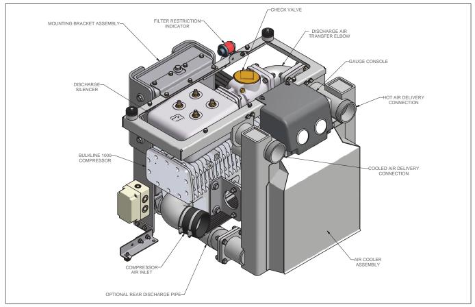
Figure 2b - Components Front Isometric View with Enclosure Removed Clockwise (Right Hand) Rotation
