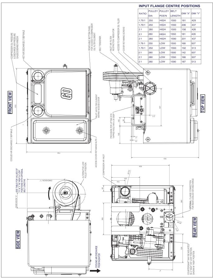
Figure 3c - General Arrangement Drawing - BL1000 Clockwise (Right Hand) Rotation Package (Pulley Shown in High Position)
