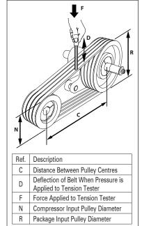
Figure 12. Belt Tension Testing
