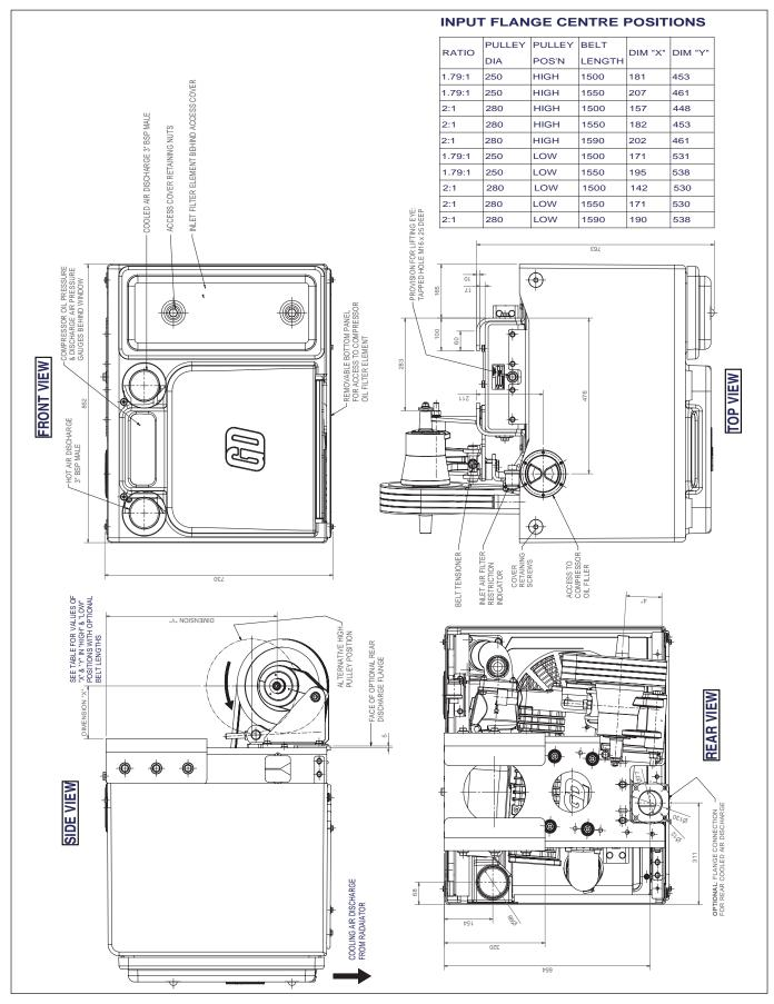
Figure 3d - General Arrangement Drawing - BL1000 Anti-Clockwise (Left Hand) Rotation Package (Pulley Shown in Low Position)
