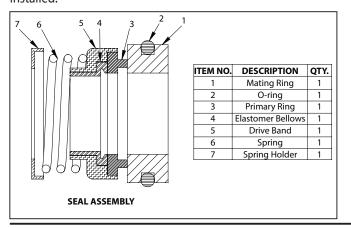
inspect the lapped sealing face of carbon washer (Part 3) for wear which would necessitate replacement.
