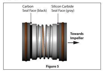
Install seal spring over drive sleeve onto backside of silicon carbide seal. Apply P80 to interior seal bellows of carbon seal and push over drive sleeve with seal pusher carbon face up. Inspect and wipe clean, if necessary. Install gasket over studs onto seal housing. Apply P80 to seal seat bore of adapter and around O-ring on seal seat. Push seal seat, by hand, into seal bore – clean and inspect.
