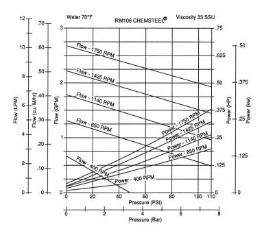
Notes: For continuous service: Plastic / Plastic gear combinations are limited to 50 psi. Metal / Plastic gear combinations are limited to 100 psi.
