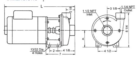
\*"L" Dimension for Single phase motors is 18 1/2"; for Three phase motors, it is 17 1/2"
