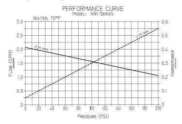
The rotary gear pump features an all bronze design and 303 stainless steel shafts with options of non-metallic gears and a variety of shaft seals. The built-in relief valve is available in multiple options; internal recirculation to suction side or external connection for return line to supply tank.
