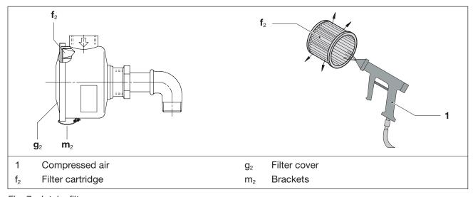
Fig. 7 Intake filter
