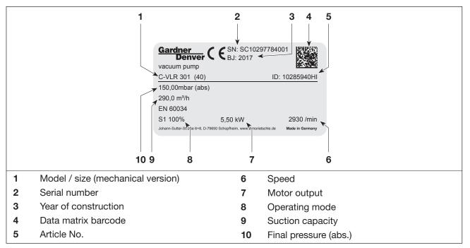
Fig. 3 Data plate (example)
