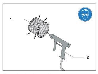
Fig. 5 Purging filter cartridge
