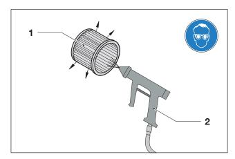
Fig. 6 Purging filter cartridge
