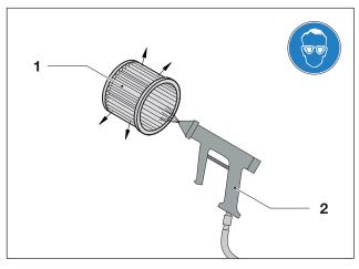
Fig. 8 Purging filter cartridge
