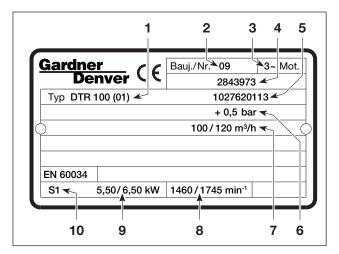
Fig. 3 Data plate (example)
