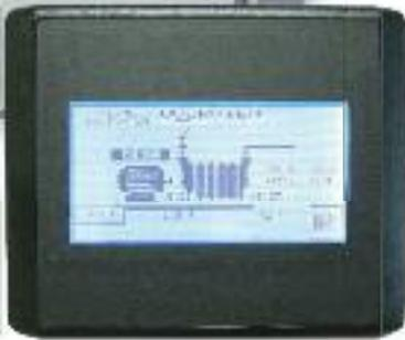
The MultiGard II is a pre-configured, programmable logic controller (PLC) capable of monitoring various operating conditions. It can even be used to monitor multiple blowers provided that there are only a limited number of variables to monitor. MultiGard II can also network with other MultiGard II controllers or be configured to various protocol systems.
