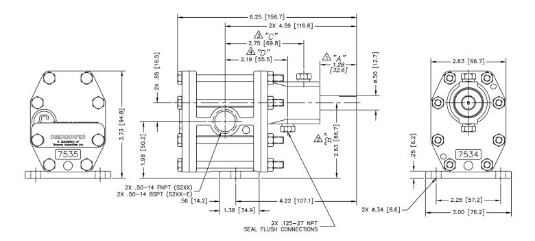
DIMENSION "A" IS APPROXIMATELY .72 [18.2] FOR PACKING PUMPS WITH PACKING NUT INSTALLED. DIMENSION "A" IS 1.26 [32.0] FOR LIP SEAL PUMPS.
