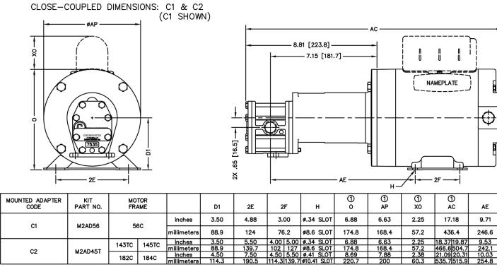
① These dimensions vary depending on hp, enclosure, speed and motor manufacturer. Specifications are subject to change without notification.
