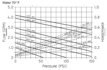
\* For pressures over 100 psi, the above selections are suitable for pumping fluids with lubricity (eq. oils, polymers). Service life will decrease for fluids without lubricity (eq. water, solvents
