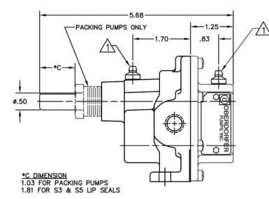
1 GREASE FITTINGS (ITEM 17) INSTALLED INTO THESE CONNECTIONS.
