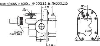
GREASE FITTINGS (ITEM 17) INSTALLED INTO .125-27 NPT CONNECTIONS.
