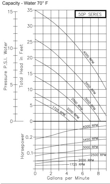
The liquid flow is proportional to the pump speed--the higher the speed the greater the flow. Horsepower required varies directly as flow and pressure. Maximum horsepower is required with a wide open discharge line. This is the point of maximum flow. With a throttled discharge, the flow decreases at a greater rate than the pressure increases thereby requiring less horsepower at the higher pressures. This is known as an "unloading" feature of the pump.
